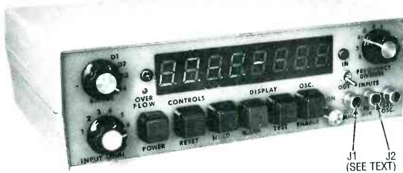
FIG. 6—THE FINISHED FREQUENCY COUNTER, shown in display-test mode, with all digits and decimal points lit. J1 and J2 are wired together, but one is unnecessary (see text).
